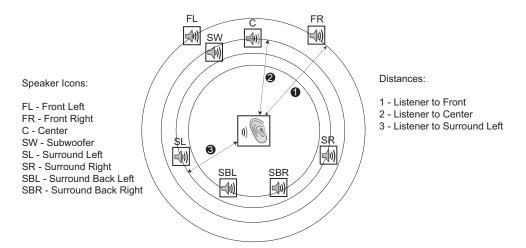
In the above diagram, measure the distance (in feet) from the primary listening position to the Front Left or Front Right Speaker. Enter the distance of the Front Speakers (**0** in the above picture) into the "Speaker Configuration" menu.
