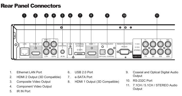
In addition to the above connectors, the AC power inlet is also located on the rear panel. The inlet is the IEC60-320 C18 type. Only the included AC power cord or an approved power cord with an IEC60-320 C17 type plug should be used.
