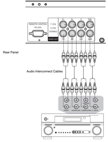
Receiver/Amplifier with 7.1ch Audio Input
