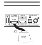
The OPPO BDP-93 Blu-ray Disc Player is equipped with two USB ports (one on the front panel and the other on the back) and one e-SATA port on the back. You may use the USB port to plug in a USB drive, or the e-SATA port to plug in an e-SATA drive.
