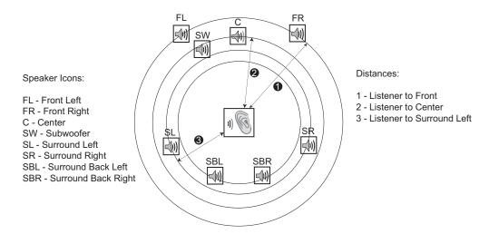
For example, in the above diagram, measure the distance (in feet) from the primary listening position to the Front Left or Front Right Speaker. Your Front Right and Left speakers should measure the same distance. If they do not, please adjust them if possible. Enter the distance of the Front Speakers (1) in the above picture) into the "Speaker Configuration" menu.
