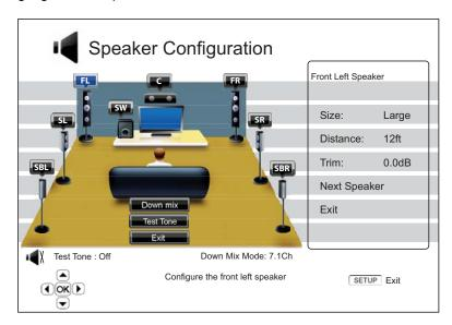
**Speaker Configuration** applies to the multi-channel analog audio outputs only. All digital bitstream and LPCM outputs are unaffected by these settings.
