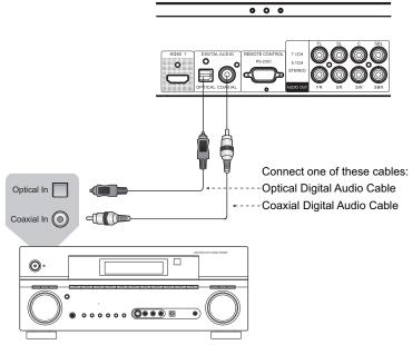
Receiver/Amplifier with Dolby Digital or DTS Decoder
