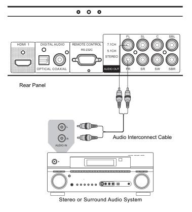
Method 7 – Stereo Analog Audio Connection
